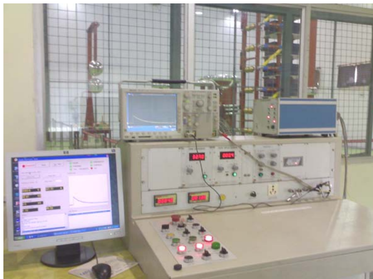
Figure 2: Control module and GUI of the impulse test setup.
