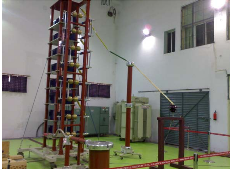
Figure 1: Hardware of the impulse voltage test setup.
